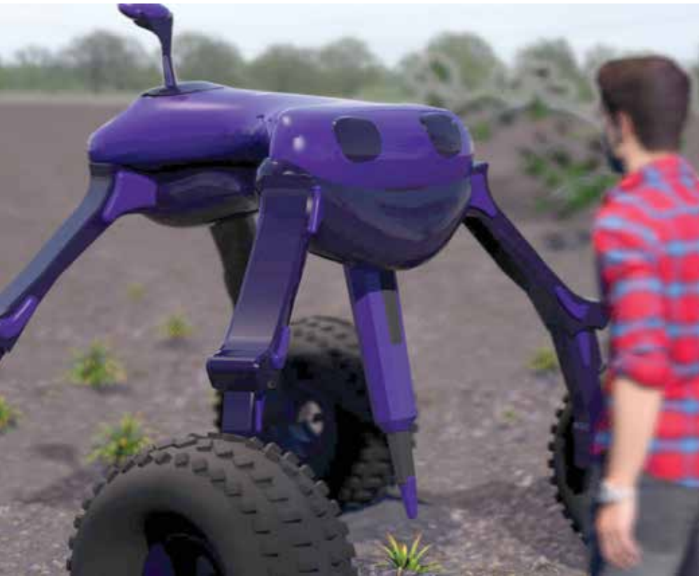
This robot from the Small Robot Company micro-sprays each plant with fertilisers or chemicals as required (Photo: Small Robot Company)
